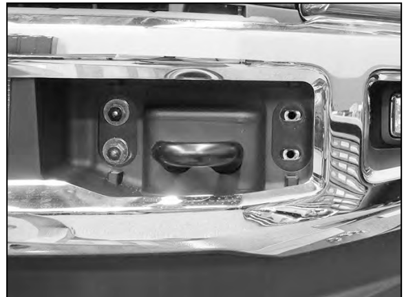
(Fig 2) Remove outer bumper bolts only
