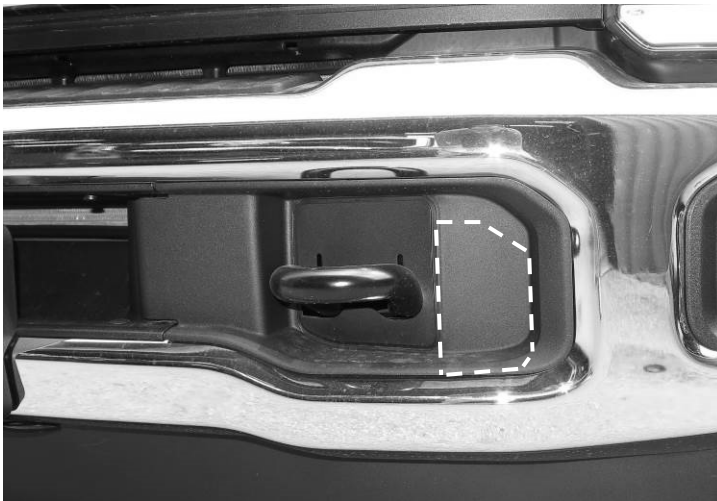
(Fig 1) Remove cover over bumper bolts.
