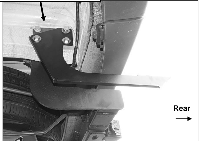
(Fig 5) Passenger side Bracket installed on outside of driver side frame channel (models with hitch only)
