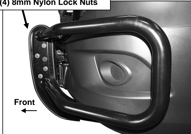
(Fig 11) Bolt Wing to Center Section (optional)
