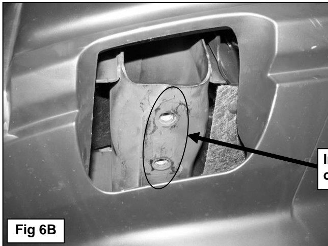
(Fig 5) Remove bumper pads to access splash guard hardware if necessary. 2017 F150 pictured
