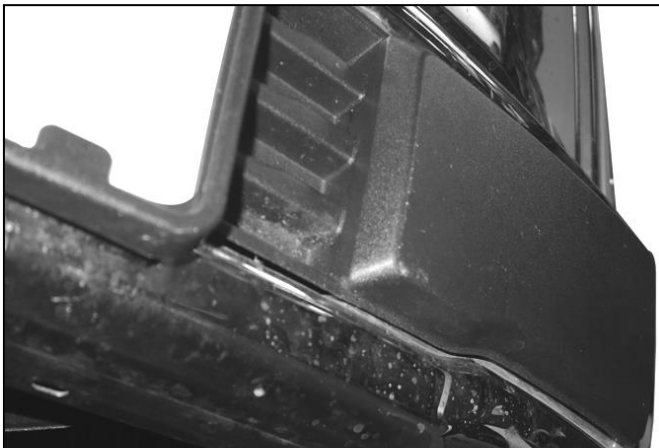
(Fig 5) Remove bumper pads to access splash guard hardware if necessary. 2017 F150 pictured
