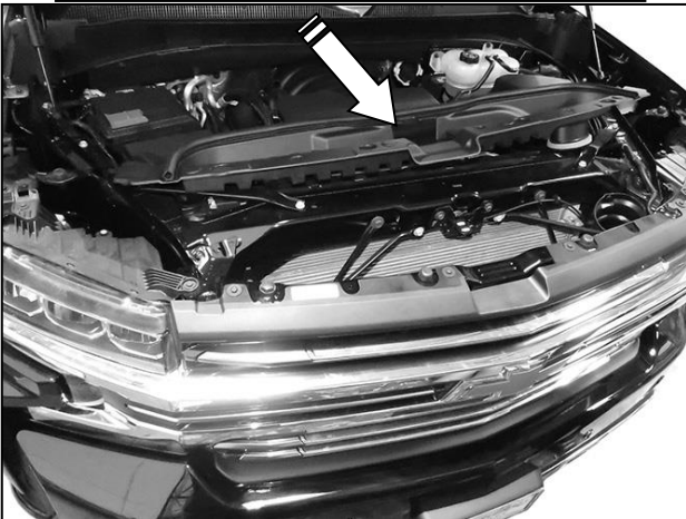
(Fig 6) Turbo Charged (gas and diesel models) with tow hooks only. Remove cover from top of radiator and grille, (arrow), Remove screws/hardware attaching grille and pull grille to release clips
