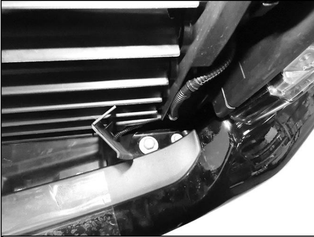
(Fig 10) Turbo Charged (gas and diesel models) with tow hooks only. Pull back cover to locate and remove bumper bolts from above
