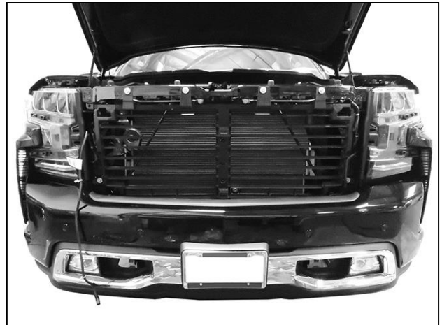
(Fig 7) Turbo Charged (gas and diesel models) with tow hooks only. Firmly pull grille straight out from vehicle
