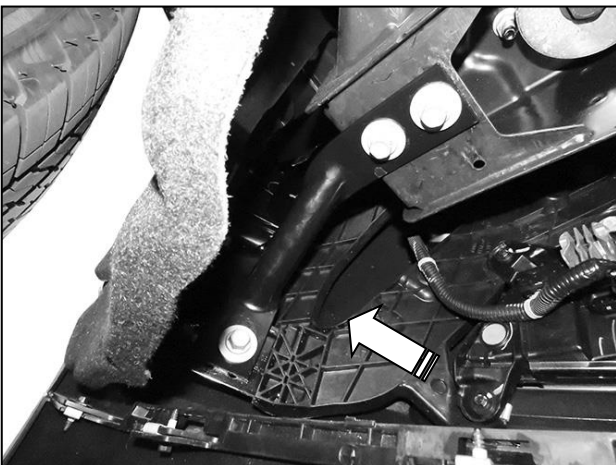
(Fig 8) Turbo Charged (gas and diesel models) with tow hooks only. Remove outer bumper supports (arrow)
