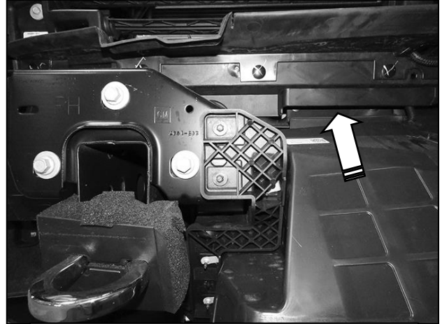
(Fig 11) Turbo Charged (gas and diesel models) with tow hooks only. Remove the bolts and pins attaching the shutter to the vehicle. NOTE: The pins are located under the plastic cover (arrow)
