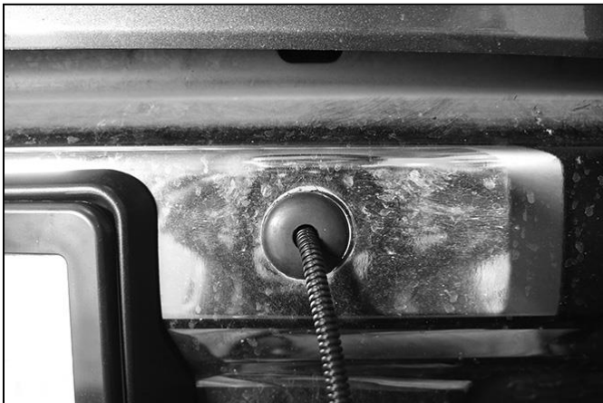
(Fig 24) Models with sensors, slide Grommet over small end of Harness Extension. Push Grommet into hole in bumper and attach to wiring harness
