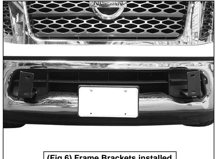
(Fig 6) Frame Brackets installed
