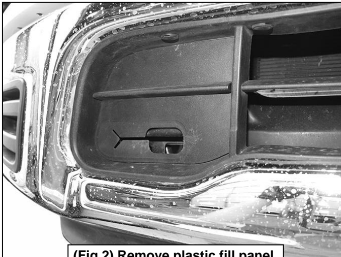
(Fig 2) Remove plastic fill panel
