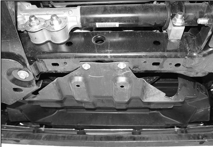
(Fig 1) Remove splash guard (pictured from below)
