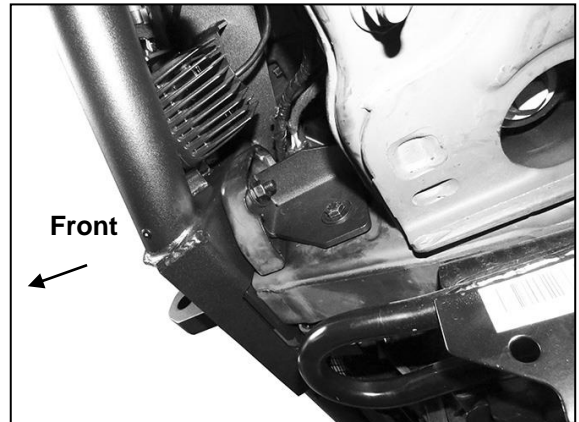
(Fig 29) Driver/left side of Bumper attached to outer Single Bolt Plate pictured from below
