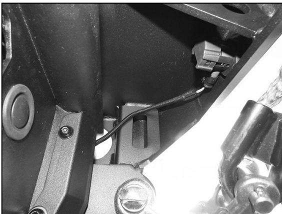
(Fig 30) Models with sensors, plug the Wiring Harness Extensions into the center sensors in the winch tray assembly (also see Fig 27). Driver/left side of winch tray pictured from below
