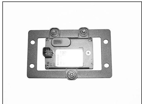
(Fig 13) ACC sensor attached to Bracket
