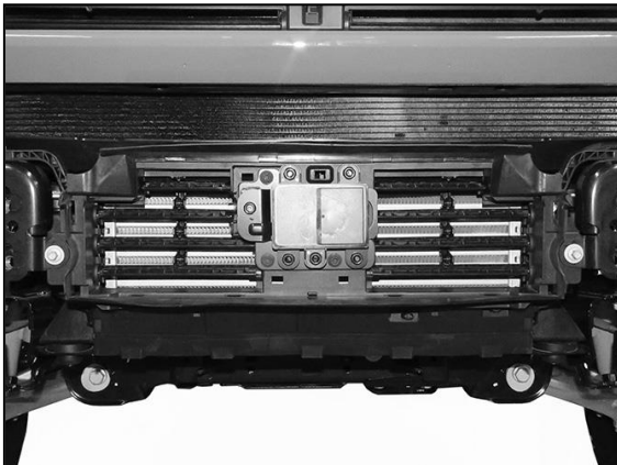
(Fig 5) Remove the shutter assembly. Models with ACC sensor (pictured), unplug and remove sensor from shutter assembly
