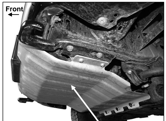
(Fig 4) Remove skid plate if equipped
