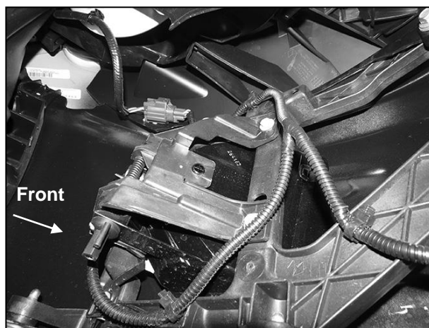
(Fig 2) Unplug lights and sensors if equipped. Unplug harness to bumper and move harness
