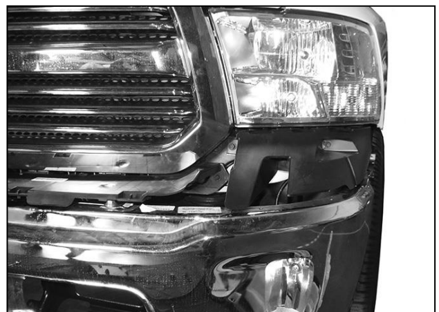
(Fig 4) Remove fascia body panel from top of bumper
