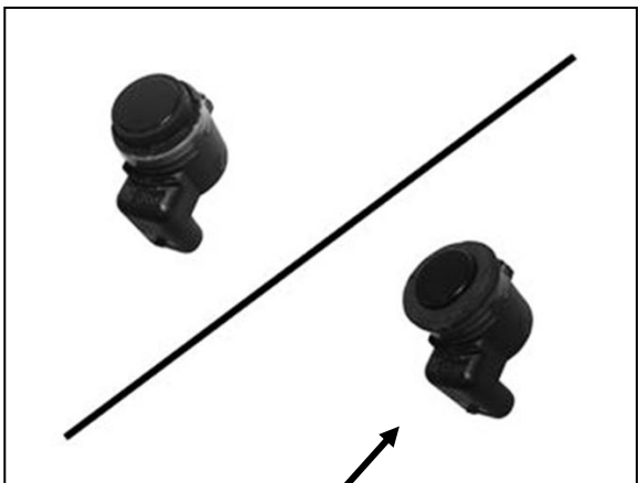
(Fig 12) Remove silicone seal from sensor. Slide large Seal over end of sensor (arrow)
