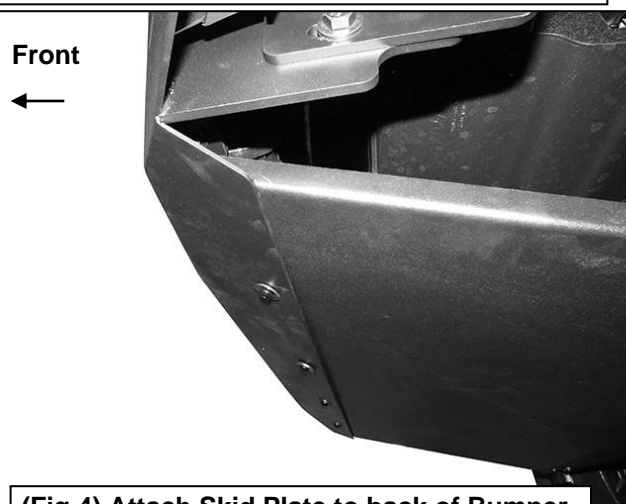
(Fig 4) Attach Skid Plate to back of Bumper
