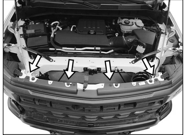
(Fig 6) Remove hardware attaching top and bottom of grille. Firmly pull grille straight out from vehicle
