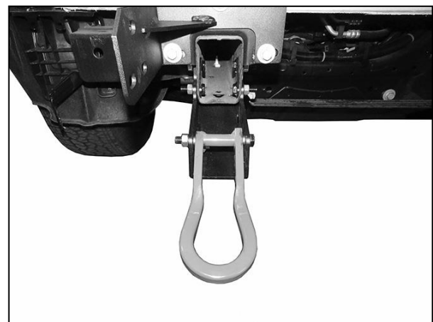
(Fig 17) Passenger/right side tow hook attached to Extension Bracket
