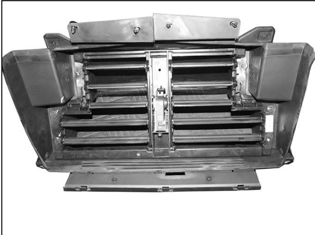
(Fig 4) Remove the shutter assembly from the outer housing
