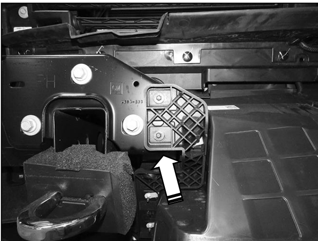
(Fig 3) Remove the bolts and pins attaching the shroud to the vehicle (arrow). Unplug and remove shutter assembly
