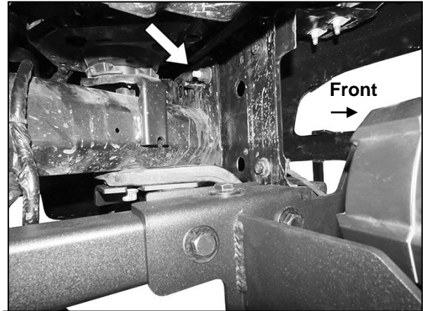
(Fig 20) Remove hex nut attaching factory bumper (arrow)
