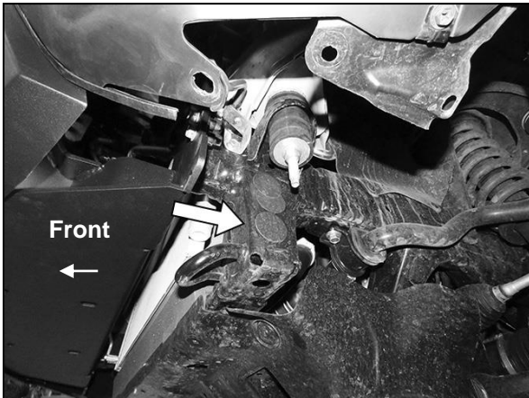
(Fig 16) Remove tape covering threaded hole in end of crossmember (arrow). Driver/left side pictured from below
