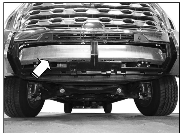
(Fig 4) Remove lower cover from bumper
