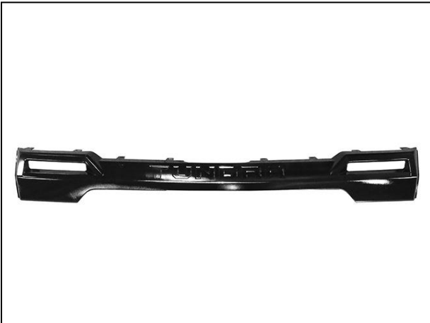
(Fig 5) Remove center body panel (fascia)
