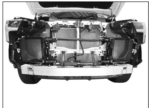
(Fig 8) Grille/bumper cover assembly removed
