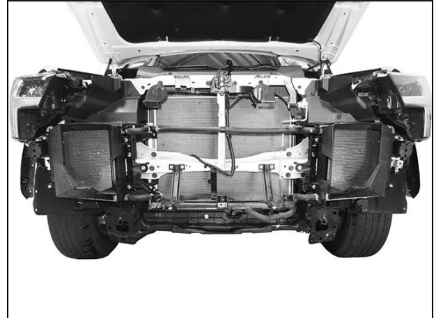
(Fig 11) Bumper, grille and impact bumper removed
