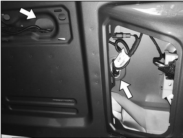
(Fig 17) Remove the plastic covers from the rear door. Feed Light Harness along the factory harness and out through the rubber plug in the door (arrows).
