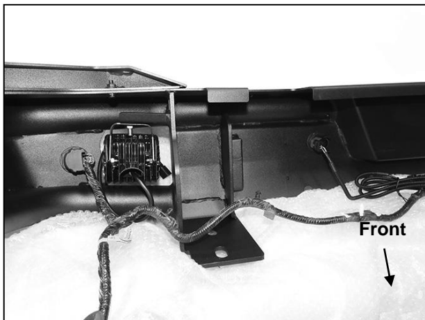
(Fig 8) Attach factory wiring harness to Bumper. Plug harness into sensors if equipped
