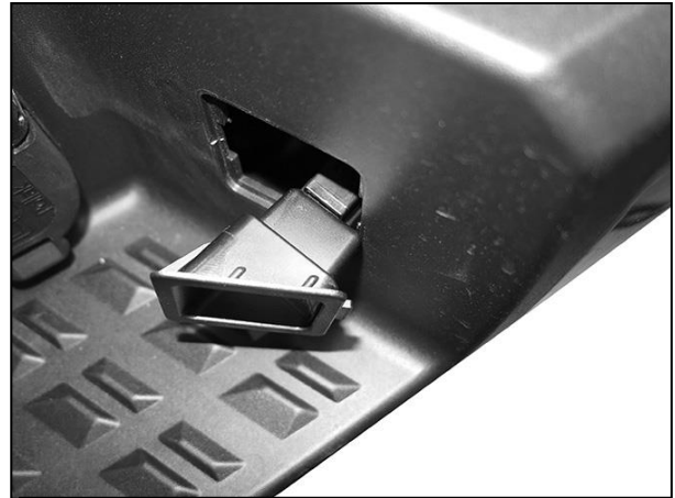
(Fig 8) Unplug and remove wiring harness, license plate lights and trailer connector
