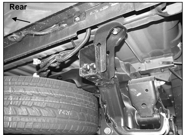
(Fig 4) Bumper completely removed, model without receiver hitch pictured
