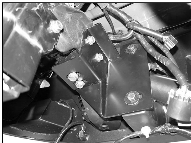
(Fig 14) Passenger/right side attached w-hitch
