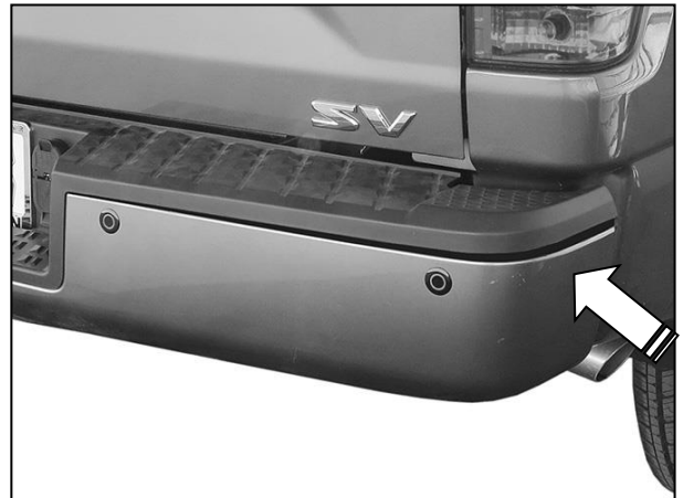
(Fig 2) Release clips attaching top cover
