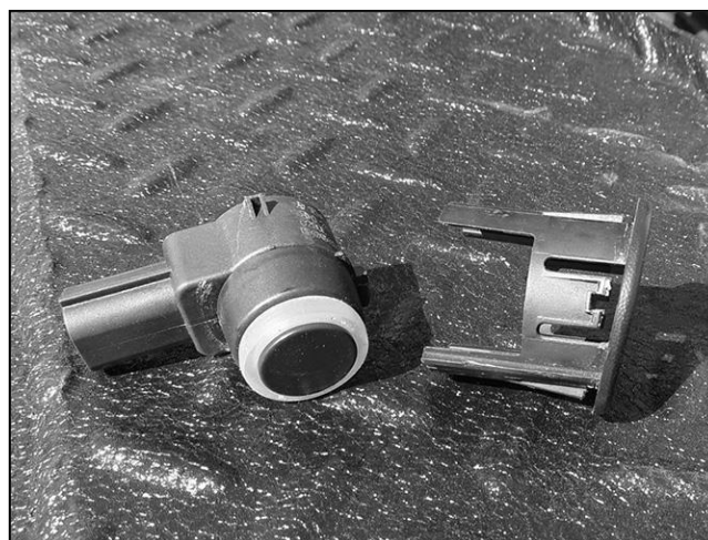
(Fig 9) Remove the sensor from the mount (right) . Remove seal from end of sensor. Push Foam Seal onto end of sensor (Fig 10)
