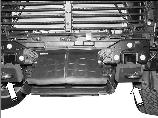
(Fig 11) Turbo Charged (gas and diesel models) with tow hooks only. Partially remove the shutter assembly to remove tow hooks and hardware (arrows)
