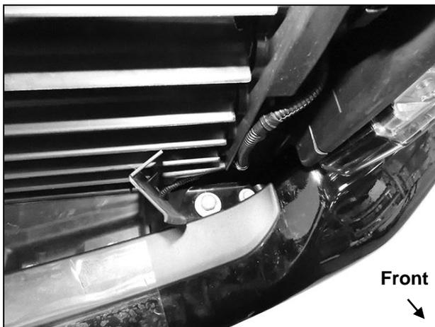
**(Fig 9) Turbo Charged (gas and diesel models) with tow hooks only.
