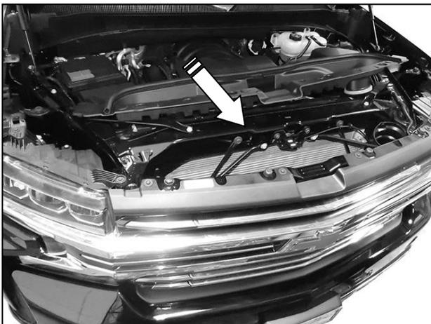
**(Fig 5) Turbo Charged (gas and diesel models) with tow hooks only. Remove cover from top of radiator and grille, (arrow), Remove screws/hardware attaching grille and pull grille to release clips**
