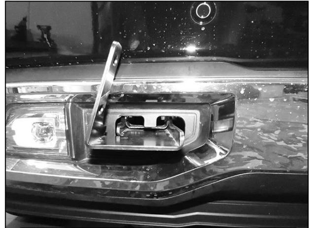
**(Fig 14) Passenger/right Bracket installed**
