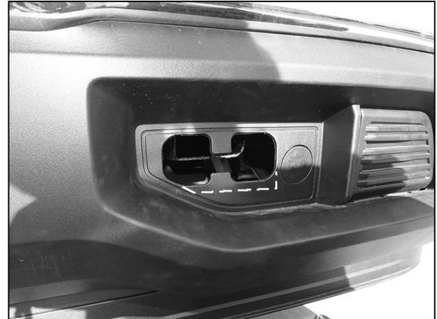
**(Fig 4) Tow hook removed. Bottom of opening may need to be trimmed to clear the Mounting Bracket**
