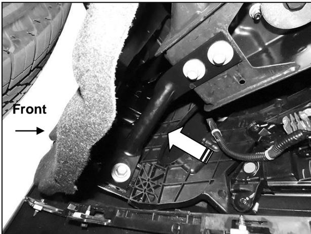
**(Fig 7) Turbo Charged (gas and diesel models) with tow hooks only.
