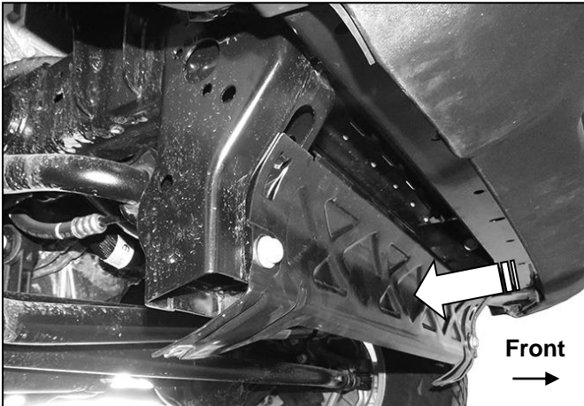
(Fig 1) Remove splash guard and bracket (arrow)
