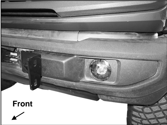
(Fig 6) Models with plastic bumper cover (see Fig 1), check for clearance between plastic cover and Mounting Bracket.
