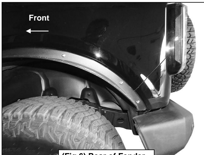
(Fig 6) Rear of Fender attached to the vehicle
