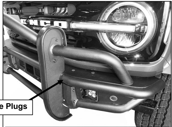
(Fig 8) After Push Bar is aligned, adjusted and all hardware fully tightened, reinstall U-Covers
