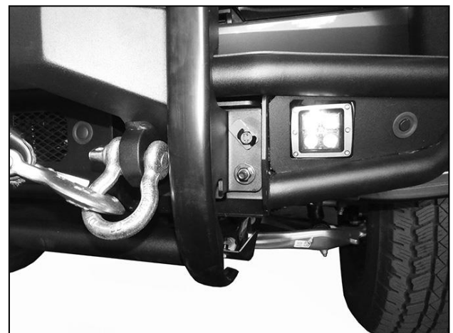
(Fig 4) Driver/left side of Push Bar attached to Bumper
