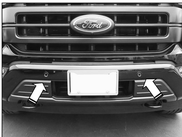
(Fig 3) Remove bumper if necessary to remove both center sensors (arrows).
