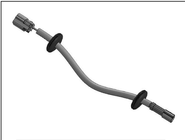
(Fig 6) Slide (2) Rubber Grommets onto Wire Harness Extension
