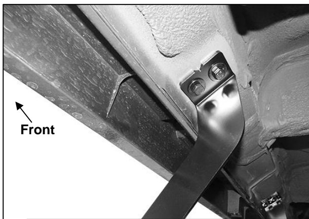
(Fig 5) Passenger/right #2, #3 and Rear Bracket attached to the #2 location
