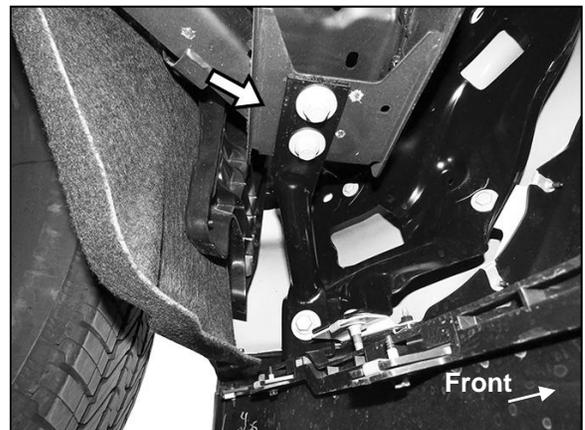
(Fig 31) 2022-on model bumper removal for tow hook reinstallation. Remove outer bumper supports (arrow). Driver/left side pictured.
