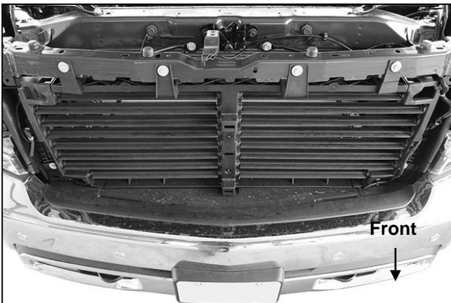
**(Fig 9) Remove screws attaching grille and carefully pull grille straight out to remove grille**
