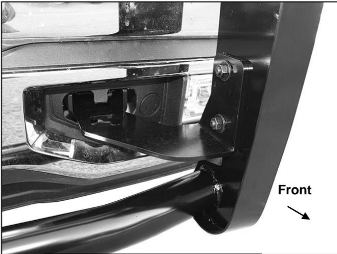
(Fig 39) Grille Guard attached to driver/left Frame Bracket
