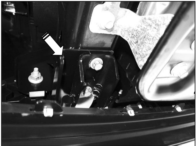
(Fig 7) Attach the driver/left Frame Mounting Bracket to the bottom of the frame. Reinstall tow hook (if equipped) over the Bracket
