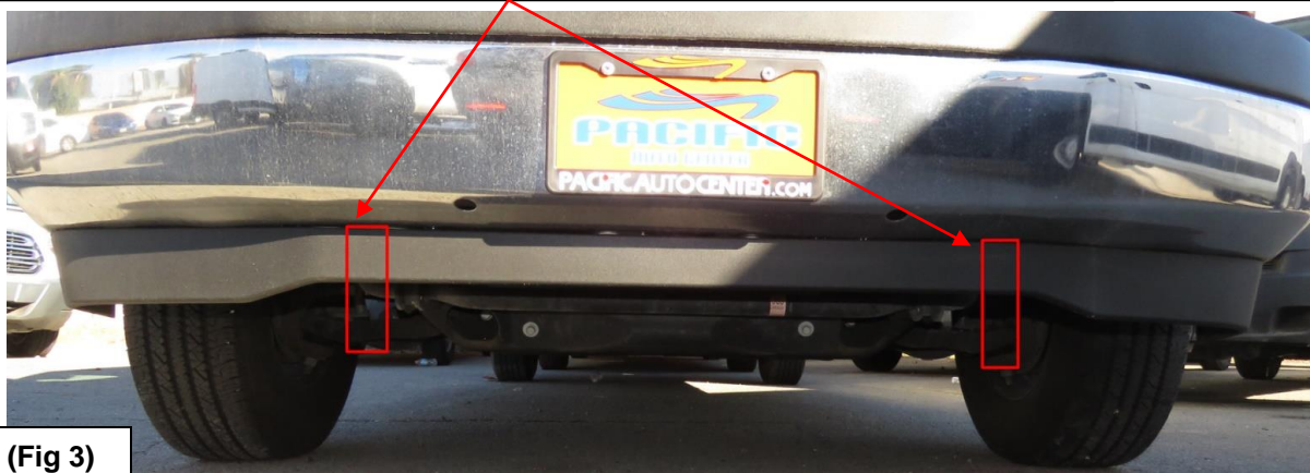
Approximate trimming locations for the air dam if end-user wants to keep it.
