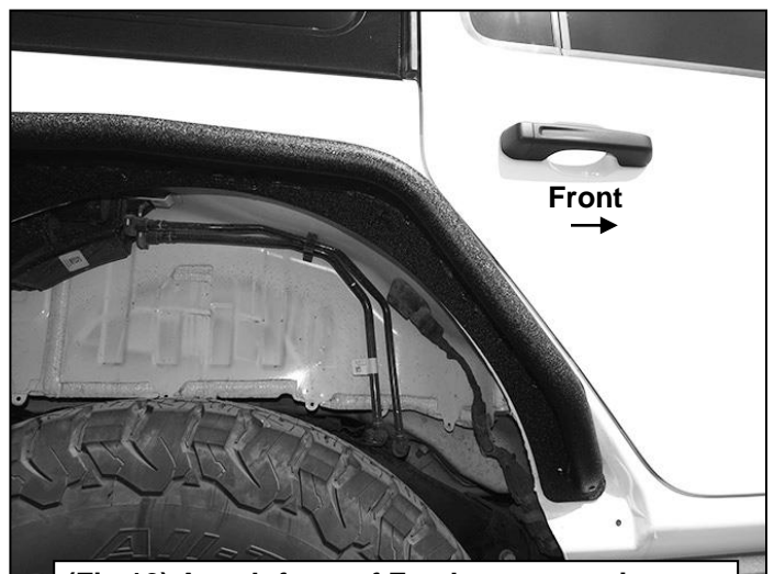
(Fig 12) Attach front of Fender to mounting locations on body, (passenger/right Fender
