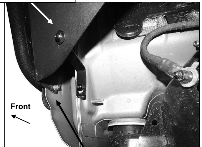
(Fig 15) Attach rear of Fender Liner to "Z" Support Bracket (Fig 7). Attach Liner to back of body panel and fender with the fender hardware or the included (1) 6mm Combo Bolt if long enough
