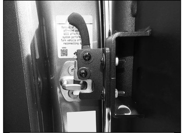
(Fig 16) Make sure door latch fully closes against striker before tightening hardware
