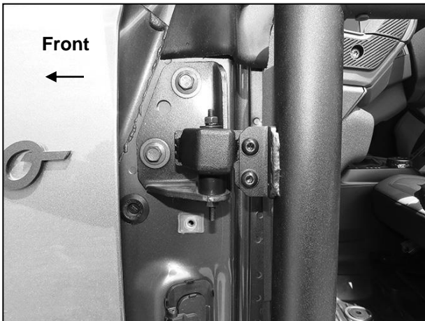
(Fig 17) Tighten hardware on Hinges (driver/left Upper Hinge pictured)
