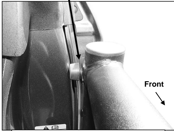
(Fig 13) Adjust Door in or out as needed
