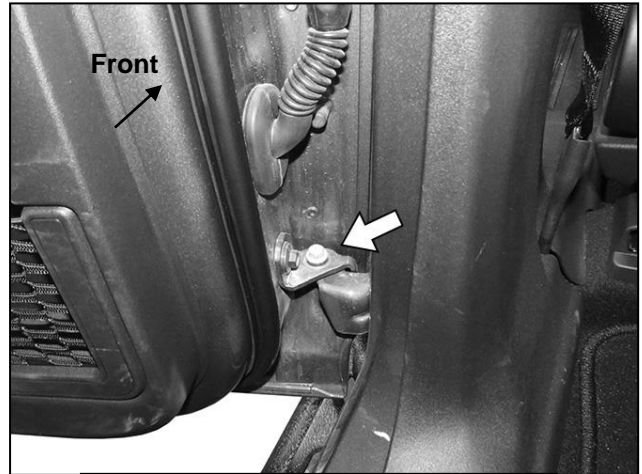
(Fig 2) Remove hardware attaching door to vehicle (arrow)
