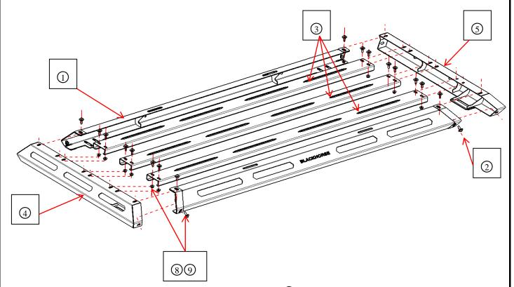
Step2: Connect the roof basket with ARMOUR II roll bar with 6 connecting bracket, then Lock all the standard
