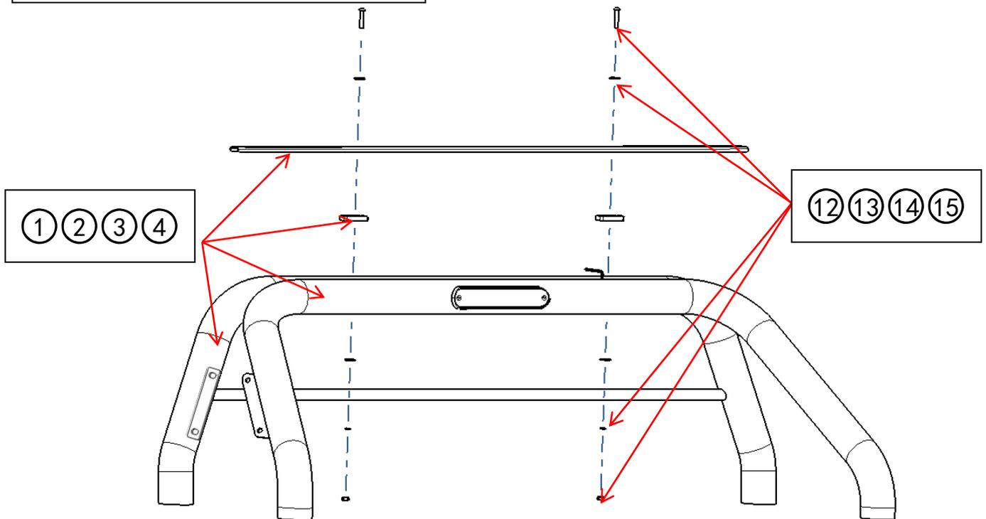
**Step2:** Assemble decoration plates and brackets with pipes. Lock all the standard parts after adjust the position.
