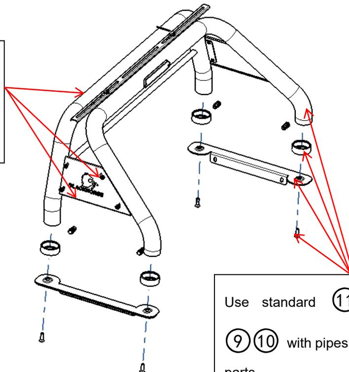
Use standard ⑪ to connect ⑨ ⑩ with pipes, 2 holes in both parts.
