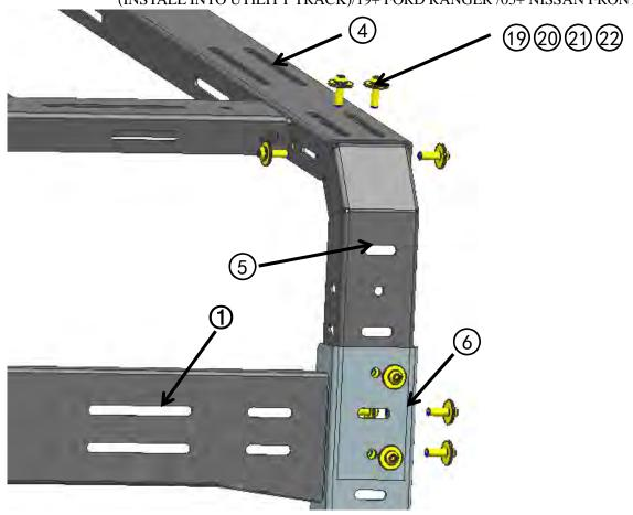
Step 5.1 (FRONTIER): Slide Nut plates 8 in the truck, and then use hardware 3 2 4 6 to connect 9 with 8. Use hardware 3 2 4 5 to install 9 with 6/7, do not tighten all the hardware.
