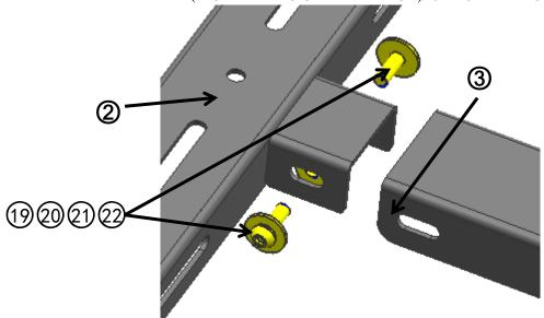
Step 3: Using hardware 19202122 to connect Cross beam 4 and Longitudinal beam 2.
