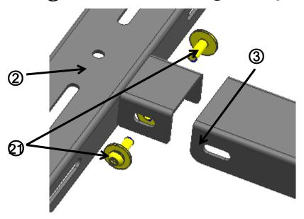
Step 3: Using hardware 21 connect Cross beam 4 and Longitudinal beam 2.
