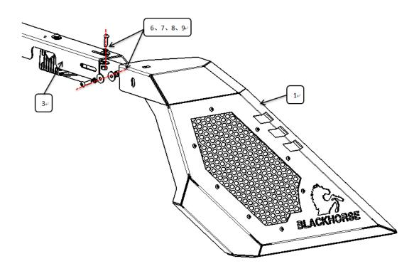
Step 3: Connect brackets and roll bar with standard parts 16 19 19 as figure shows.
