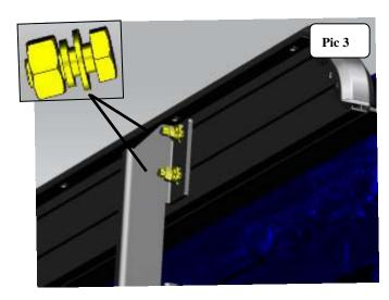
Step 4: Refer to Pic 3 to install V1 Running Board with running board hard ware.
