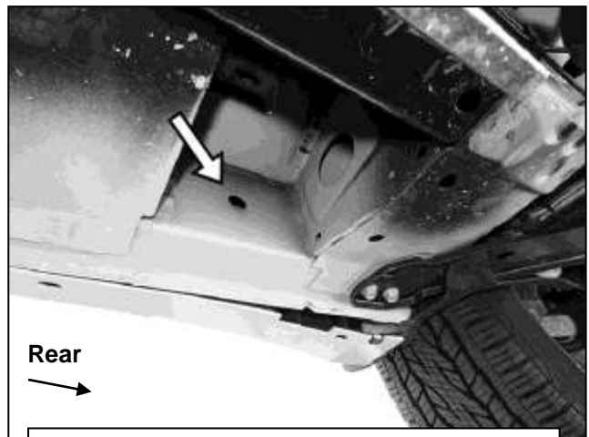
(Fig 13) Remove plug from Passenger/Right rear mounting location
