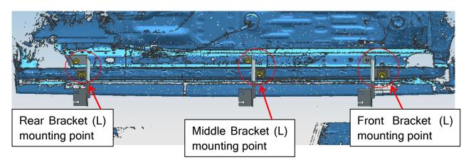
Step 2: Attach Front Bracket (L) ①, Middle Bracket (L) ③ and Rear Bracket (L) ⑤ on the mounting points with T Bolts M10x40 ⑦, Plastic Retainers φ10 (δ0.7\*40\*40) ⑥, Hex Nuts M10 ⑨, Flat Washers D10 (10x30x2.5mm) ⑫, Flat Washers D8 (8x24x2mm) ⑫, Hex Bolts M8\_30 ௰, Lock Washers D8 む and Lock Washers D10 ₺. Front Bracket (R) ②, Middle Bracket (R) ④ and Rear Bracket (R) ⑥ refer to left side installation, and the right and right sides are symmetrical.
