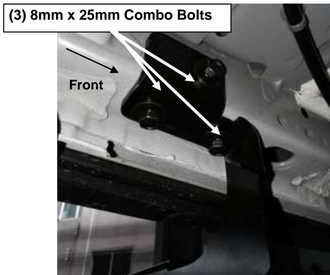
(Fig 5) Driver /Left Rear Mounting Bracket Pictured
