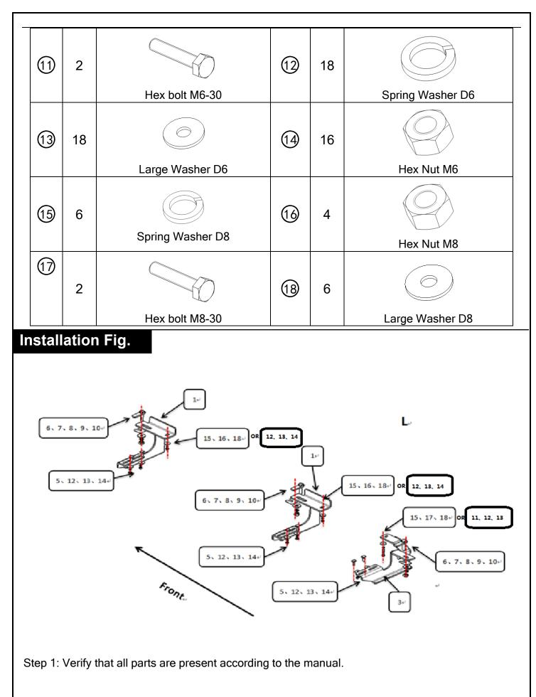
Step 2: Install the brackets and running board on the bottom of vehicle as above picture. PS:For connect bracket to the bottom of vehicle, there are two sets optional accessories parts (NO#11-14)&(NO#15-18), you could select best one to install according to actual installation.
