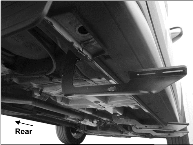
(Fig 12) All Mounting Cradles should face towards the rear
