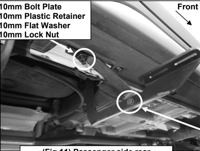
(Fig 11) Passenger side rear mounting strap and bracket installed
