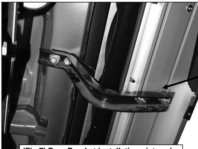
(Fig 7) Rear Bracket installation pictured
